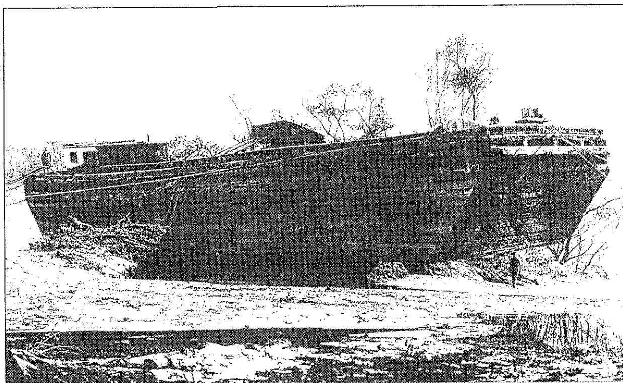
Figure 38. Typical scow-built box design (origin unknown).
