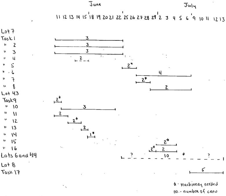
Figure 1. Projected schedule and estimated level of effort for mitigation work during the five week period of slurry wall completion.
