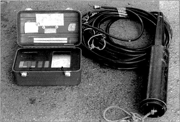
Figure 42. Geometrics 866 magnetometer.
