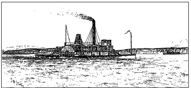
Figure 17. Representation of the *Norwich*, a 160-foot former passenger steamer employed for towing (as presented in Swanton n.d.). Note the vessel's crosshead engine.
