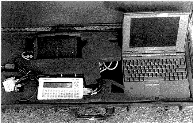
Figure 41. Motorola LGT-1000 global based navigation system.
