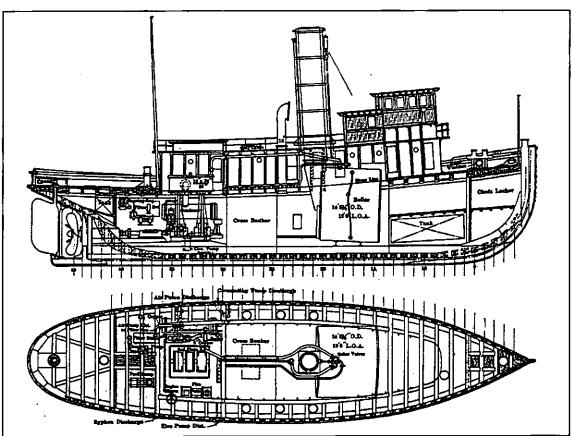
Figure 21. General plan and profile of a 100-foot wooden tug, circa 1920 (as presented in International Marine Engineering 1920).
