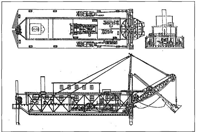
Figure 11. Inboard profile, deck plan, and cross section of the *Toledo*, a wooden-hulled bucket dredge. Note the spuds, the large legs that raise and lower and anchor the dredge in place (as presented in International Marine Engineering 1910).
